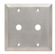
Double gang, Double telephone or cable outlet with removable 13/32 ft ID grommet in 17/32-inch hole. Box mounted. 302/304 Stainless steel.
