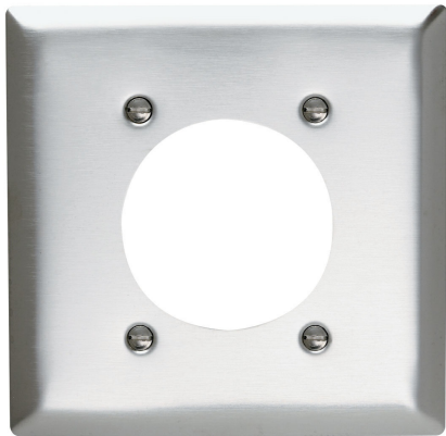
2-Gang Power Outlet Receptacle Opening, 2.1563 in hole for 2.125-inch diameter device - 4 mtg. holes, Smooth 302/304 Metal.
