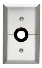
Single-Gang, Single outlet horizontal split wall plate for television or cable lead in. Supplied with #340 yoke, Strap mounted removable 5/8 ft ID grommet in 7/8-inch hole. Smooth 302/304 Stainless Steel.
