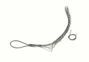
Double Weave, Standard Length, Split Lace, Offset Eye. Cable Diameter - 1.250-1.490\'\', Mesh Length - 17\'\', Break Strength -4,100 lbs.
