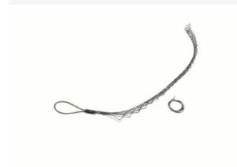
Double Weave, Long Length, Split Lace, Offset Eye. ◆ Cable Diameter - 1.250-1.490\'\', Mesh Length - 24\'\', Break Strength-4,100 lbs.
