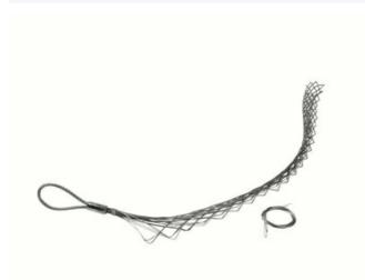
Double Weave, Long Length, Split Lace, Offset Eye. ◆ Cable Diameter - 2.000-2.490\'\', Mesh Length - 27\'\', Break Strength - 7,300 lbs.
