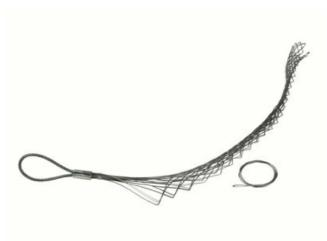
Double Weave, Long Length, Split Lace, Offset Eye. ◆ Cable Diameter - 3.000-3.490\'\', Mesh Length - 33\'\', Break Strength - 9,200 lbs.
