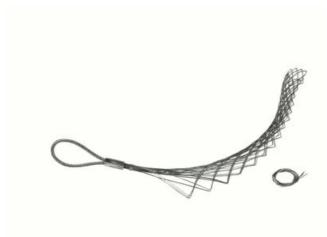
Double Weave, Standard length, Split Lace, Offset Eye. ◆ Cable Diameter - 3.500-3.900\'\', Mesh Length - 33\'\', Break Strength - 9,200 lbs.
