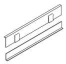
Used to separate Trenchduct and fittings into two or more compartments. Allows 3/4" (19.1mm) upward adjustment. Field installed to base and adjusted up to bottom of cover plate of Trenchduct with welds or screws. Available in 5' (1.5m) length. Field modified for use in T-Units, risers, and elbows.
