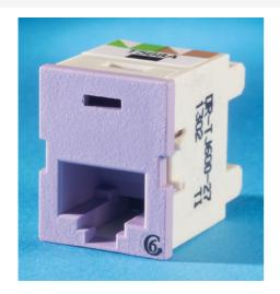
Clarity 6a, 6 & 5e TracJacks, ETL verified to TIA Category 6a, 6 & 5e component specification. Front-loading and front removable. New universal T568A/B wiring label and tapered wiring towers simplify termination. Center tuned to Clarity patch cords for optimum performance.
