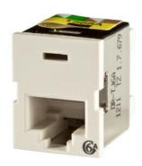
Clarity 6a TracJack, ETL verified to TIA Category 6a component specification. Front-loading and front removable. New universal T568A/B wiring label and tapered wiring towers simplify termination. Center tuned to Clarity 6a patch cords for optimum performance
