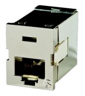
Clarity 6 Shielded, TracJack, ETL verified to TIA Category 6 component specification. Front-loading and front removable. New universal T568A/B wiring label and tapered wiring towers simplify termination. Center tuned to Clarity 6 Shielded patch cords for optimum performance.
