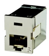
Clarity 6A Shielded, TracJack, ETL verified to TIA Category 6A component specification. Front-loading and front removable. New universal T568A/B wiring label and tapered wiring towers simplify termination.
