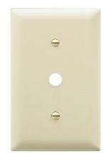
Single gang, Single telephone or cable outlet 13/32" hole. Strap mounted with adjustable yoke. One #340 yoke. Nylon trademaster plate. Vory.
