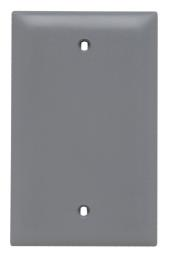
The Trademaster 1-gang blank wall plate is constructed from high-impact, injection molded nylon plastic. Oversized in height and width by 3/16<sup>ths</sup> of an inch, this plate could completely cover an opening in a wall that a standard plate fails to conceal.
