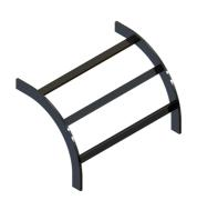
Radius curved runway permits smooth vertical to horizontal transitions. Stringers are 1-.5 in x .375 in steel tubes; cross slats are 1 in x .5 in x .125 in steel tubes. UL listed.
