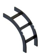
Radius curved runway permits smooth vertical to horizontal transitions. Stringers are 1-.5 in x .375 in steel tubes; cross slats are 1 in x .5 in x .125 in steel tubes. UL listed.
