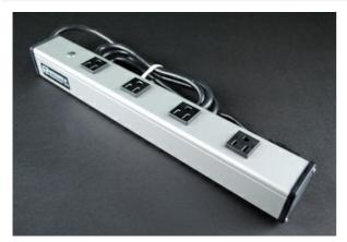
Four outlets, rugged gray aluminum housing, 15A, receptacles rotated 90 degrees and spaced to accommodate transformers. 15' [4.6m] 14/3 SJT black cord with NEMA5-15 plug. Length 16'' [406mm]. Receptacle center-to-center 3'' [76mm]. Snap-on, slide-off mounting.
