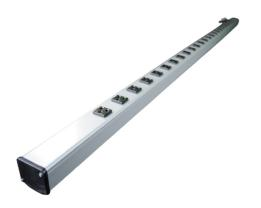
Twenty-four outlets, rugged gray aluminum housing, 15A, 15' (4.6m) 14/3 SJT black cord with NEMA5-15 plug. Length 72'' (1.8m). Receptacle center-to-center 2 1/2'' [64mm].
