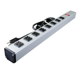
Eight outlets, lighted switch, rugged gray aluminum housing, 15A, 6' (1.8m) 14/3 SJT black cord with NEMA5-15 plug. Length 24'' (609mm). Receptacle center-to-center 2'' (51mm). Snap-on, slide-off mounting.
