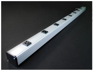
Eight outlets, rugged gray aluminum housing, 15A, 6' (1.8m) 14/3 SJT black cord with NEMA5-15 plug. Length 48'' (1.2m). Receptacle center-to-center 5 1/4'' (133mm). Snap-on, slide-off mounting.
