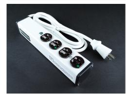
Four outlets. Rugged white aluminum housing. 15' (4.6m) 14/3 SJT white cord with NEMA5-15 plug. Length 10 3/4" (237mm). Receptacle center-to-center 1 1/2" (38mm). Snap-on, slide-off mounting. Not for use in critical care enviornments. NOTE: Not for use where Article 517 of NEC requires Hospital Grade Outlets.
