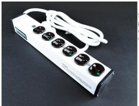
Six outlets. Rugged white aluminum housing. 15' (4.6m) 14/3 SJT white cord with NEMA5-15 plug. Length 13 1/4'' (337mm). Receptacle center-to-center 1 1/2'' (38mm). Snap-on, slide-off mounting. Not for use in critical care enviornments. NOTE: Not for use where Article 517 of NEC requires Hospital Grade Outlets.
