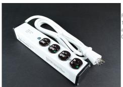
Four outlets. Rugged white aluminum housing. 15' (4.6m) 14/3 SJT white cord with NEMA5-15 plug. Length 10 3/4'' (237mm). Receptacle center-to-center 1 1/2'' (38mm). Snap-on, slide-off mounting. cTUVus Listed as Medical Electrical Equipment. NOTE: Suitable for use where Article 517 of NEC requires Hospital Grade Outlets.
