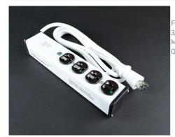
Four outlets. Rugged white aluminum housing. 6' (1.8m) 14/3 SJT white cord with NEMA5-15 plug. Length 10 3/4" (237mm). Receptacle center-to-center 1 1/2" (38mm). Snap-on, slide-off mounting. cTUVus Listed as Medical Electrical Equipment. NOTE: Suitable for use where Article 517 of NEC requires Hospital Grade Outlets.
