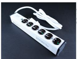
Six outlets. Rugged white aluminum housing. 6' [1.8m] 14/3 SJT white cord with NEMA5-15 plug. Length 13 1/4'' [337mm]. Receptacle center-to-center 1 1/2'' [38mm]. Snap-on, slide-off mounting. cTUVus Listed as Medical Electrical Equipment. NOTE: Suitable for use where Article 517 of NEC requires Hospital Grade Outlets.
