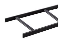
Universal Style Tubular Runway features 1 in x. 5 in tubular cross slats that are welded between  $.375 \times 1.5$  in high tensile tubular steel stringers. Cross slats feature rounded edges for cable protection. Standard length is 9ft 11 in, and widths from 6 in to 24 in. Available in rust-resistant, powder coated black finish only. UL listed.
