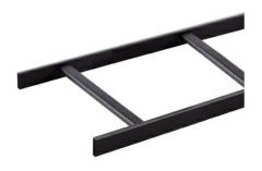
Universal Style Tubular Runway features 1in x .5in tubular cross slats that are welded between .375 x 1.5in high tensile tubular steel stringers. Cross slats feature rounded edges for cable protection. Standard length is 9ft 11in, and widths from 6in to 24in. Available in rust-resistant, powder coated black finish only. UL listed.
