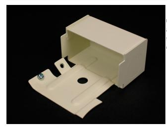
Connects 3000 Series Raceway with 1/2" trade size conduit and armored cable connectors. 1/2" trade size KOs on end and each side of fitting. Can be connected to conduit boxes by using 1/2" chase nipple.
