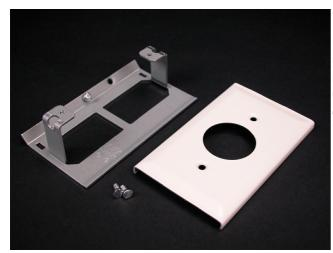
Installs commercially available straight blade and locking single receptacles with face diameters of 1.38" - 1.40" (35mm - 36mm) into 3000 Series Raceway. G3007C Device Bracket included. NOTE: Certified to Canadian Safety Standards for sale in Canada. When ordering these products, change the "V" color prefix to "CV" or the "G" color prefix to "CG" to denote the Canadian versions.
