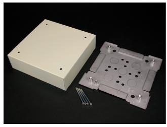
Used as a tee, cross, junction box, or for branch circuit extensions in 3000 Series Raceway. Cover has raceway twistouts on all sides. Base has five 1/2" trade size KOs and four fixture mounting holes.
