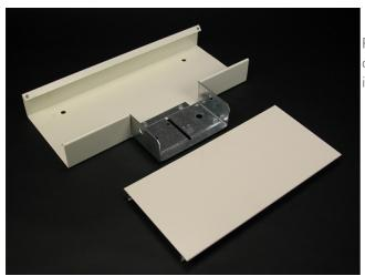
For branching raceway at right angles. Use with undivided raceway only. Join to raceway run with two pair of 4001A Couplings (not included).
