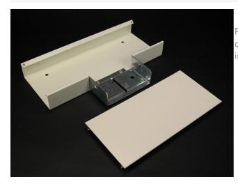
For branching raceway at right angles. Use with undivided raceway only. Join to raceway run with two pair of 4001A Couplings (not included).
