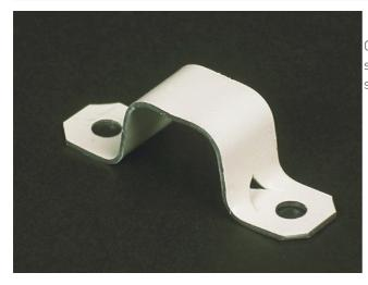
Converts to one-hole by breaking off at score. Lanced tab holds strap in place while fastening to surface. NOTE: Use #8 panhead screws.
