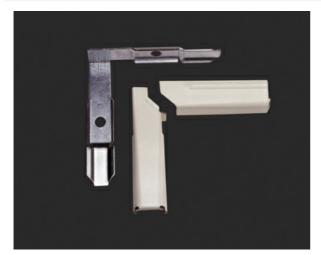
For 90 degree twist with a 90 degree turn. For double turn at right angles from one surface to another. For transitions from a sidewall to ceiling or edge of door or window trim. Twistout in cover adapts for use with 700 Series Raceway.
