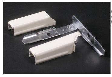
For 90 degree twist with a 90 degree turn. For double turn at right angles from one surface to another. For transitions from a sidewall to ceiling or edge of door or window trim. Twistout in cover adapts for use with 700 Series Raceway.
