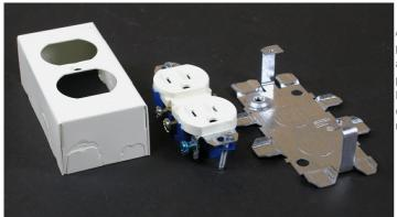
Accommodates 15A (NEMA 5-15R) or 20A (NEMA 5-20R) duplex devices in place of duplex grounding receptacle included. Cover has twistouts for 500 and 700 Series Raceway on each end and sides. Twistouts on ends of box permit running raceway close to interior trim. Base has 1/2" trade size KOs. NOTE: Certified to Canadian Safety Standards for sale in Canada. When ordering these products, change the "V" color prefix to "VC" to denote the Canadian versions.
