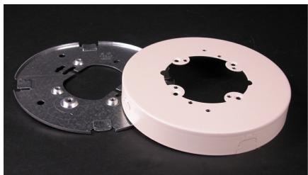
Mounts onto 3 1/4" or 4" (83mm or 102mm) conduit boxex, or other recessed outlets. Cover accepts devices with mounting screw centers of 2 3/4", 3 1/2", or 4 1/16" (70mm, 89mm, or 103mm). Can be used with 5736 Blank Cover as a pull or junction box. Outside diameter 6 3/8" (162mm).
