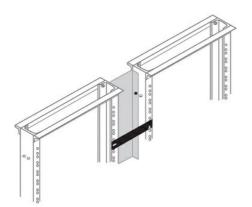
Vertical control brackets attach to equipment racks to provide secure backside cable containment; Legrand recommends using four brackets on an 84" rack.
