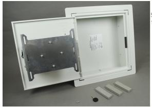
5" deep enclosure for 2' x 2' drop ceiling tile with faceplate for mounting CISCO Aironet 1250 and 3500 Series using remote antennas, 13" W x 14" L (330mm x 356mm).
