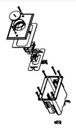
Includes single-gang box, device plate with two openings for communication devices, and nickel cover with one screw plug. For hole cut dimensions, see installation instructions sheet. Box Dimensions: 2 1/8" W x 3 3/4" L x 3 7/8" D (54mm W x 95mm L x 98mm D) Device Plate: 3 1/8" W x 4 15/16" L (79mm W x 125mm L).
