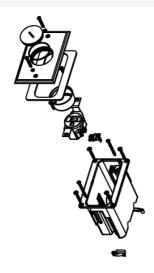
Includes single-gang box, one 15A tamper-resistant receptacle, and nickel cover with one screw plug. For hole cut dimensions, see installation instructions sheet. Box Dimensions: 2 1/8" W x 3 3/4" L x 3 7/8" D (54mm W x 95mm L x 98mm D) Device Plate: 3 1/8" W x 4 15/16" L (79mm W x 125mm L).
