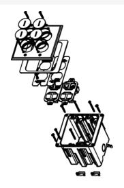
Includes dual-gang box, two 106 adapter with eight openings for communication devices, and brass cover with four screw plugs. For hole cut dimensions, see installation instructions sheet. Box Dimensions: 3 1/4" W x 3 3/4" L x 3 7/8" D (83mm W x 95mm L x 98mm D) Device Plate: 4 7/8" W x 5 1/16" L (124mm W x 129mm L).
