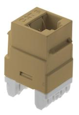
Ensure high-performance network connections with this Cat 6 RJ45 Keystone Connector in ivory. The standard RCA front jack connects to Cat5, Cat5e, or Cat6 cables terminated with RJ-45 plugs. The vertical design makes punchdown termination easy, while rear retention caps ensure secure wire connections. It meets Category 6 standards described in TIA/EIA-568-B.2.
