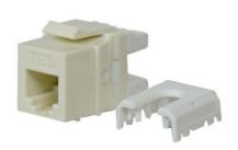
Part of the Quick Connect family of products, this RJ25 keystone insert supports up to three telephone lines and accepts an RJ45 plug without damage. Easily terminate all four pairs using the Legrand Punch & Go Tool (AC3400). With 50 microinches of gold on contacts, this insert ensures reliable and high-quality connections. The QuickConnect termination reduces installation time, making it an efficient choice for your network setup. It is also FCC Part 68 compliant.
