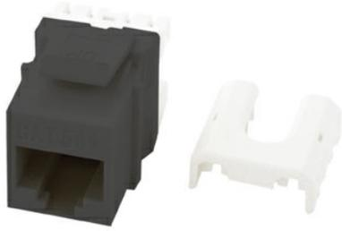
The Cat 5e Quick Connect RJ45 Keystone Insert in light almond is designed for efficient and reliable network connections. This insert is ETL Verified to the Category 5e component standard, ensuring compliance with industry standards. It can be terminated with any 110 punchdown tool and exceeds EIA/TIA 568A/B Cat 5e Performance Specifications. Available in multiple colors, this insert is perfect for various networking applications.
