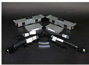
Kit contains three 4-wire, 2 circuit connectorized cables, two 12" in length (one M/F and one F/F) and one 17" (F/F), all with black cable covers and 8 cable clamps for mounting. Also two work surface portals each with 2 power outlets accessible from table surface and 2 convenience power outlets accessible from under the table, 2 keystone openings for communications and one silver flange cover. Portals are wired for circuit 1. For circuit 2 wired portals, order the "-2" suffixed part number.
