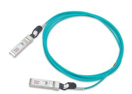
30m Intel XXVAOCBL30M Compatible 25GBase-AOC SFP28 to SFP28 (MMF, 850nm, LSZH) Active Optical Cable
