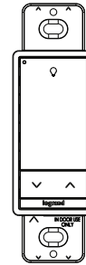
Remove all wings to wall box mount using a Decora cover plate
