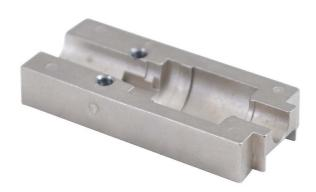
The Visual Fault Locator (VFL) Test Adapter for Simplex SC Infinium Mechanical Fiber Connectors allow the visible indicators in the Infinum mechanical fiber connector to be viewed when using a VFL to ensure cable continuity and determine a pass or fail termination.
