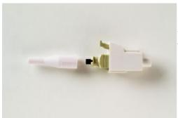
Legrand quick-cure, anaerobic epoxy field-installable connectors speed installation time. Strip the fiber, inject the adhesive into the connector, insert and scribe the fiber, then polish the connector end face to perfection for a high performance termination.
